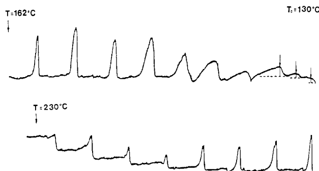
Figure 1. Thermogram of a solution of polydisperse PE sample (Marlex) in 2,4-dimethylpentane showing the photocell signal at each temperature increment \Delta T_i between 130 and 240 °C. The \Delta T_i vary from 2 to 9 °C as the MW diminishes. The thermocouple recordings have been deleted from the figure for clarity. The sets of h_i(T_i) are as listed in the Appendix. The turbidity signals for the first three peaks have been marked. For that particular thermogram, the second and third \Delta T were effected before the return of the transmitted light to the base line. The h_i are not changed if one waits longer between the peaks.
